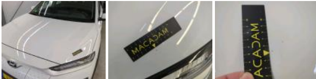
Bumper moulding F, Scratch(es), Replace and paint
