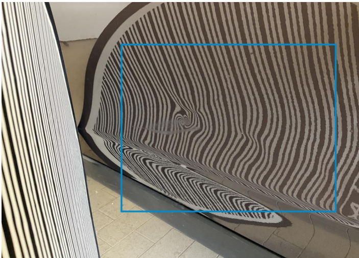
5. Door / Front Left Bodywork / Breakage / Crack -
