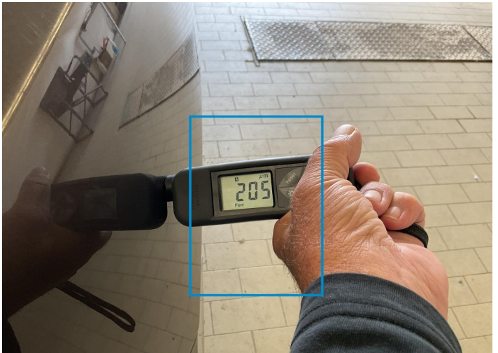
14. Fender / Front Left Paint / Poor Previous Repair -
