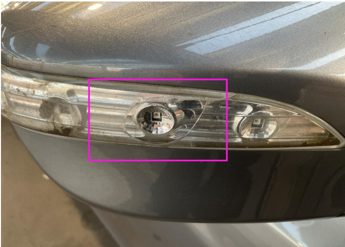
4. Mirror Repeater / Right Glass Break -
