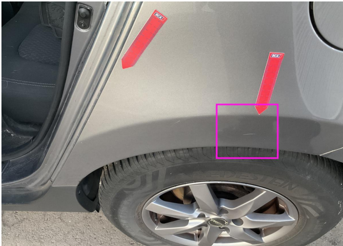
3. Fender / Back Right Paint / Scratch / Scuff -
