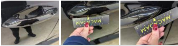
Door RL, Scratch(es), Repair and paint (complete)
