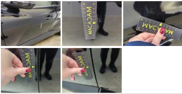
Outer door handle FL, Scratch(es), Repair and paint (complete)
