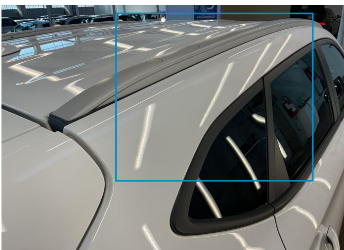
4. Pillar / Front Right Bodywork / Poor Previous Repair -
