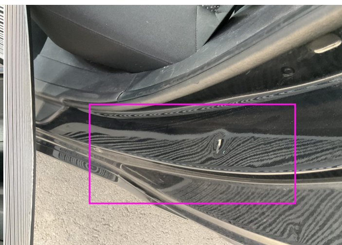
16. Rocker Panel / Center Left Bodywork / Dent / Dent -
