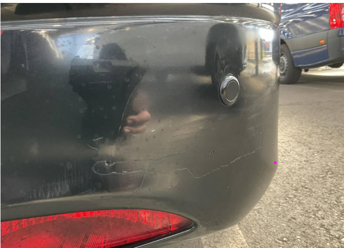
29. Bumper / Back Paint / Poor Previous Repair -
