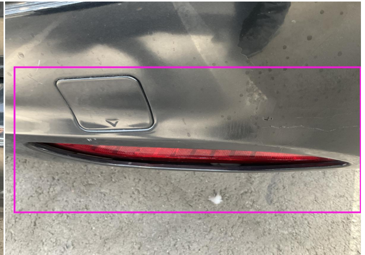
28. Bumper / Back Bodywork / Breakage / Crack -
