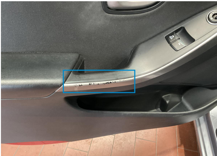
5. Interior door handle Front left Interior / Scratched -
