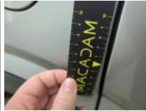
Door FR, Scratch(es), Repair and paint (complete)
