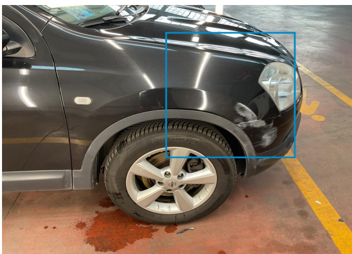
15. Fender / Front Right Bodywork / Dent -
