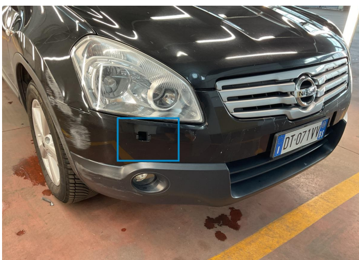
17. Headlight Nozzle / Front Right Missing Part -
