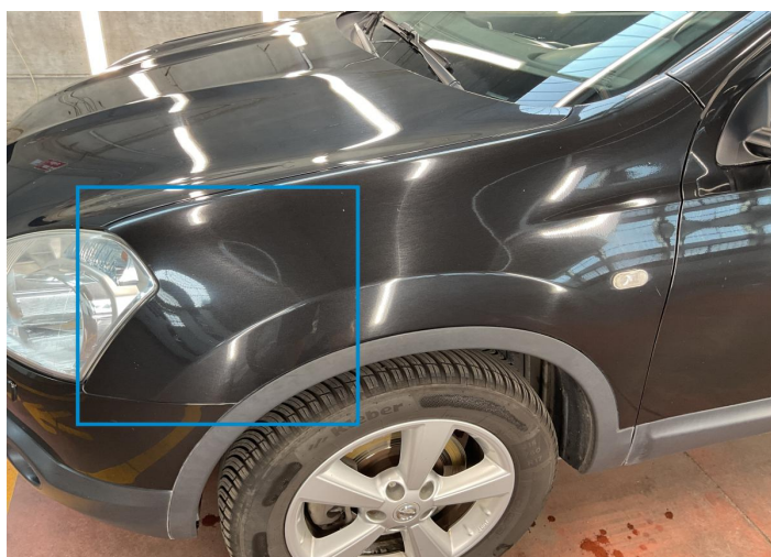
21. Fender / Front Left Paint / Chipping -
