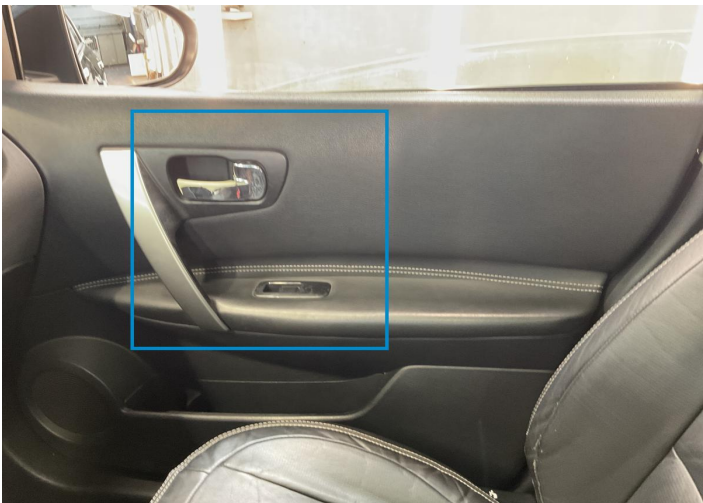
2. Panel Filling / Front Right Interior / Worn - out -
