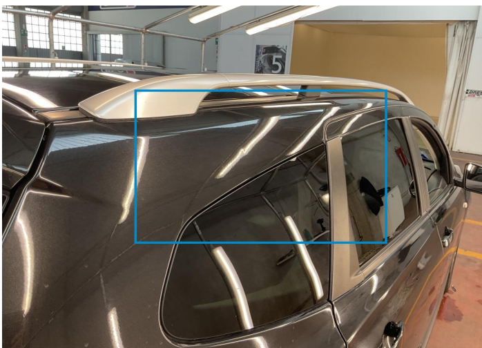
35. Pillar / Front Right Bodywork / Dent / Hail Area -
