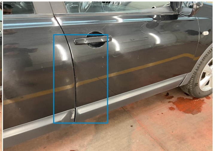
34. Door / Front Right Bodywork / Dent -
