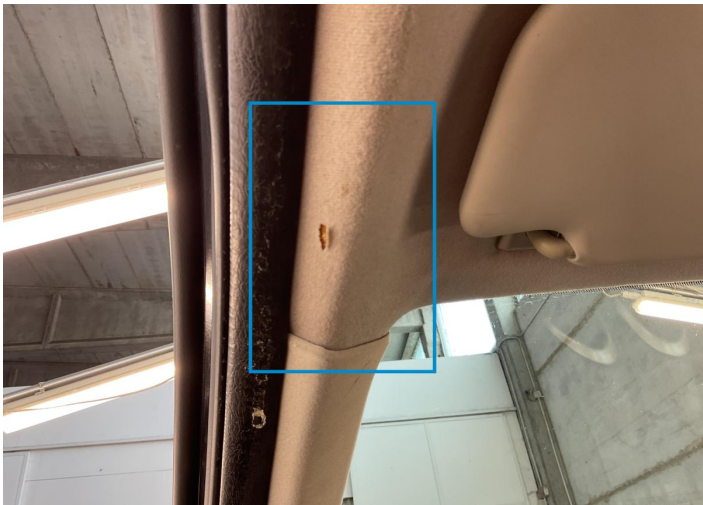
5. Roof Upholstery Interior / Ripped -
