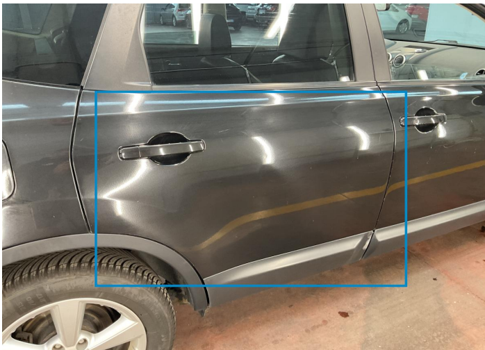
33. Door / Back Right Bodywork / Poor Previous Repair -
