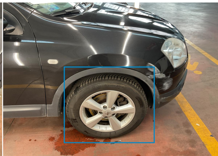
14. Rim / Front Right Out of Bodywork / Scratch -
