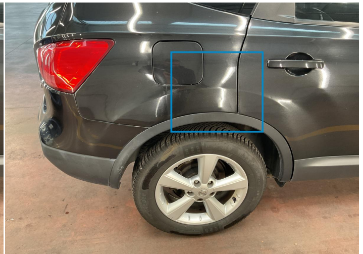
32. Fender / Back Right Bodywork / Dent -
