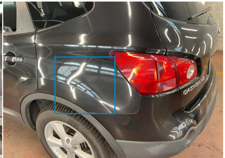
26. Fender / Back Left Bodywork / Dent -
