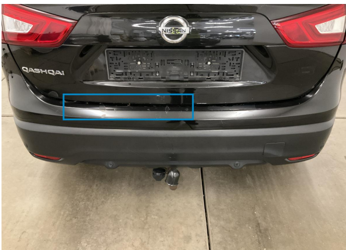
12. Bumper / Back Paint / Poor Previous Repair -
