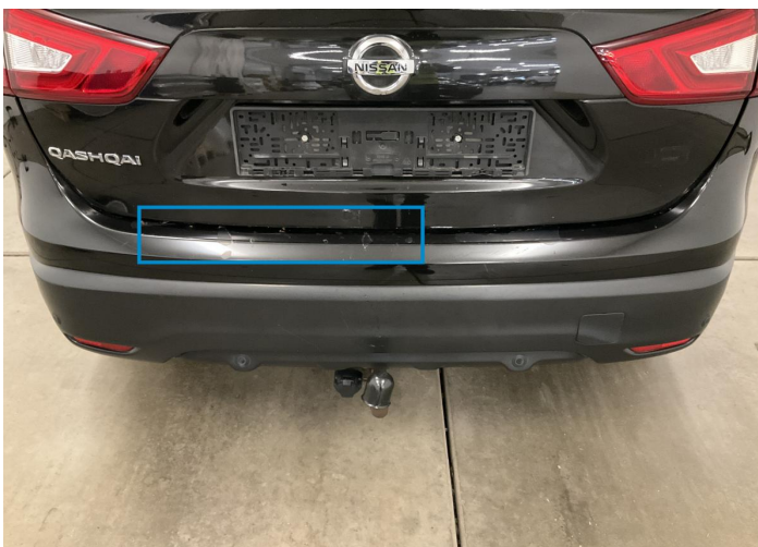
12. Bumper / Back Paint / Poor Previous Repair -
