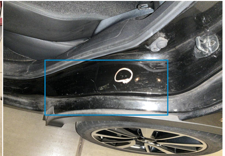
14. Pillar / Back Left Bodywork / Dent / Dent -
