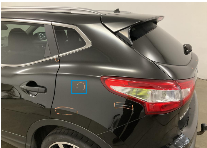
1. Side Panel / Back Left Bodywork / Dent / Dent -
