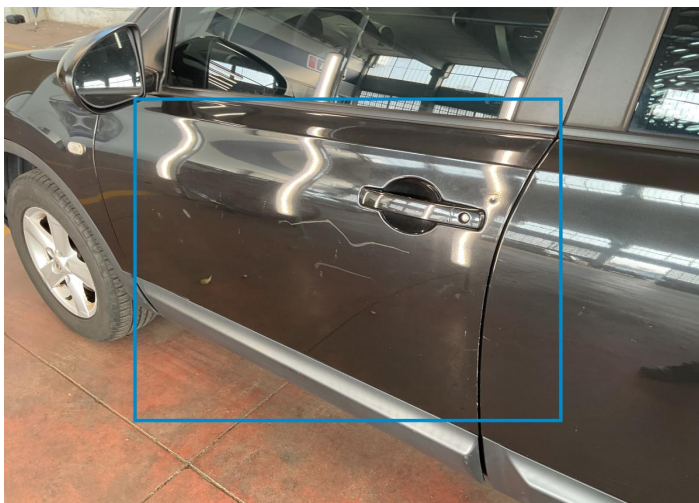
9. Door / Front Left Bodywork / Dent -
