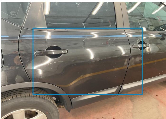
10. Door / Back Right Bodywork / Dent -
