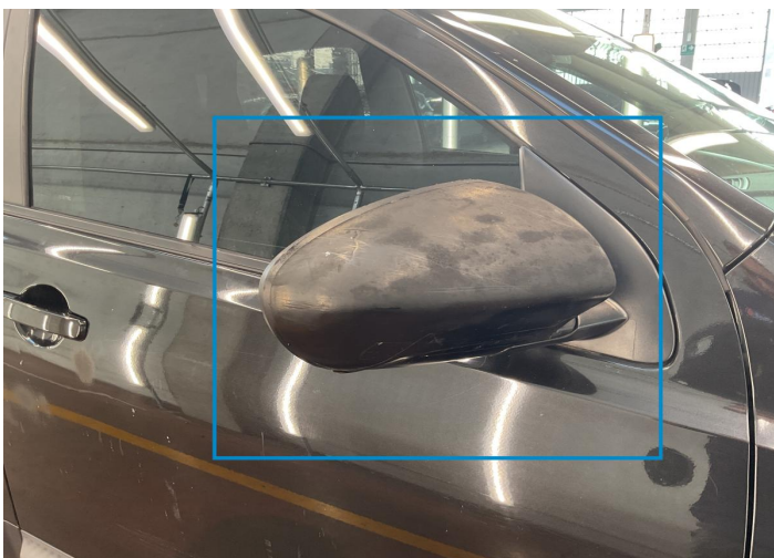
12. Mirror Shell / Front Right Bodywork / Breakage -
