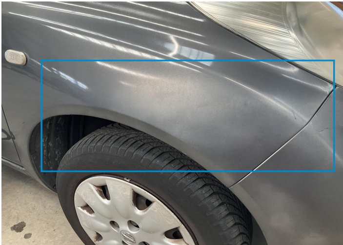
27. Fender / Front Right Paint / Poor Previous Repair -
