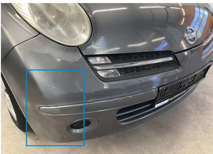
2. Bumper / Front Paint / Poor Previous Repair -
