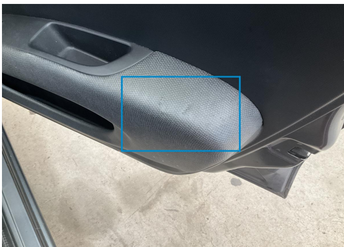
23. Panel Filling / Front Right Interior / Scratched -
