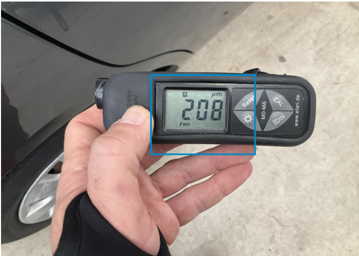
28. Fender / Back Right Paint / Poor Previous Repair -
