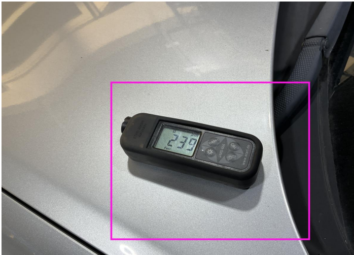
3. Door / Front Left Paint / Poor Previous Repair -
