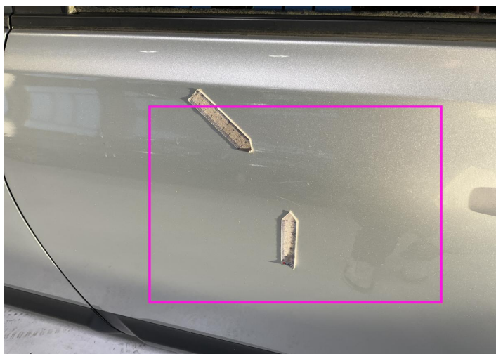
19. Door / Back Left Paint / Scratch / Scuff -
