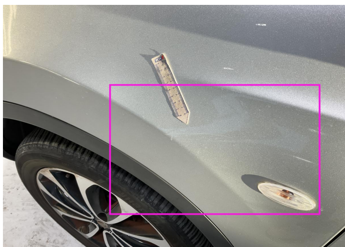
21. Wing Expander / Front Left Paint / Scratch / Scuff -
