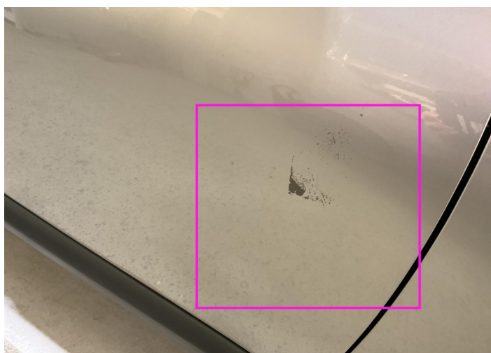
7. Door / Front Right Paint / Scratch / Scuff -
