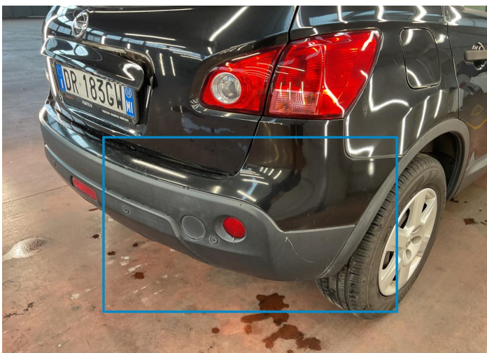
26. Bumper / Back Paint / Scratch / Line -
