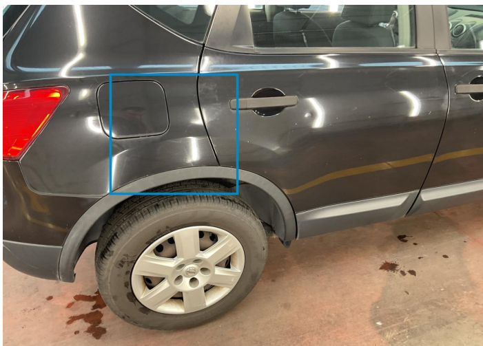
27. Fender / Back Right Bodywork / Dent -
