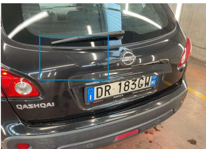
24. Tailgate Paint / Scratch / Line -
