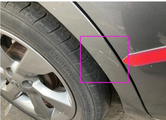
29. Fender / Back Right Paint / Scratch / Scuff -
