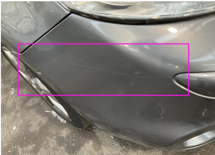
17. Corner Bumper / Front Right Paint / Scratch / Scuff -
