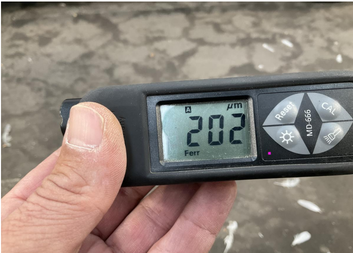
10. Door / Back Right Paint / Poor Previous Repair -
