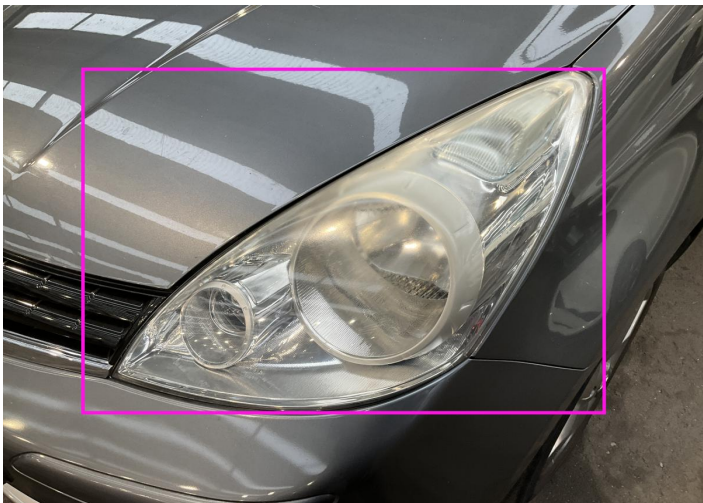
13. Front Light / Front Left Glass Break -
