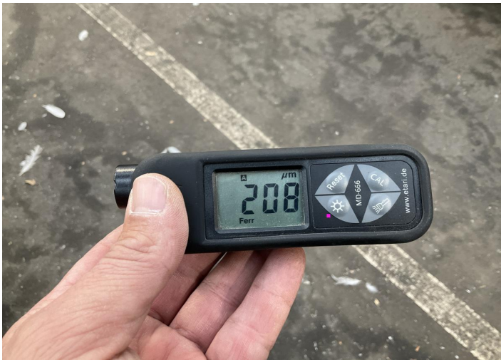
11. Door / Front Right Paint / Poor Previous Repair -
