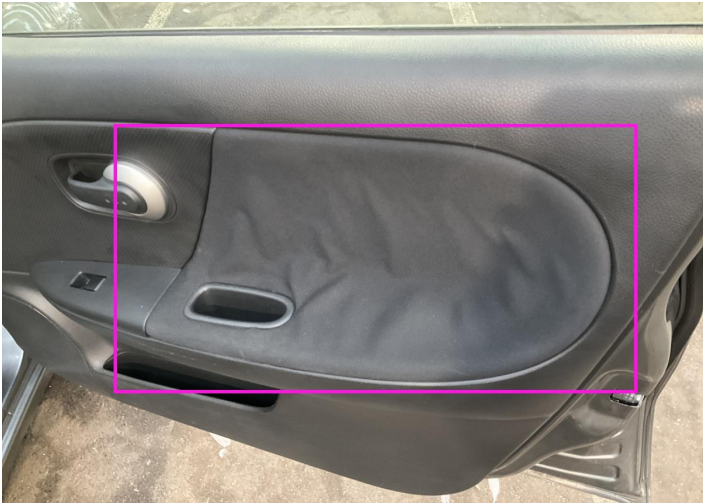
6. Panel Filling / Front Right Interior / Loose -
