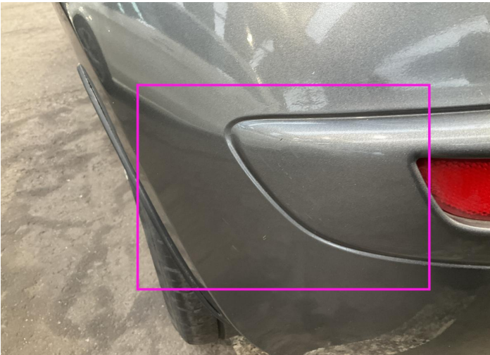
25. Corner Bumper / Back Left Paint / Scratch / Scuff -
