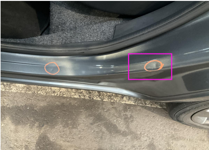
4. Pillar / Back Left Bodywork / Dent / Dent -
