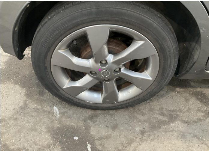
27. Rim / Back Right Out of Bodywork / Scratch -
