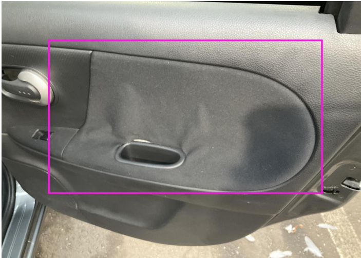
5. Panel Filling / Back Right Interior / Loose -
