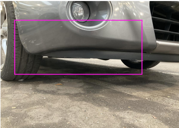
18. Corner Bumper / Front Right Paint / Scratch / Scuff -
