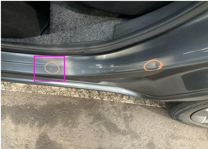
3. Pillar / Back Left Bodywork / Dent / Dent -
