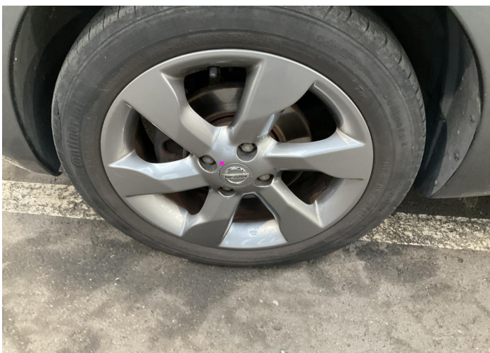
20. Rim / Front Left Out of Bodywork / Scratch -
