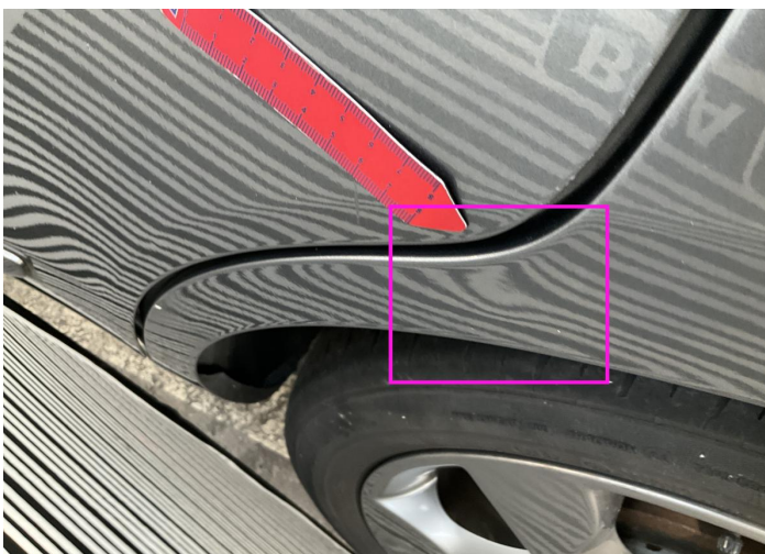
24. Fender / Back Left Bodywork / Dent / Dent -
