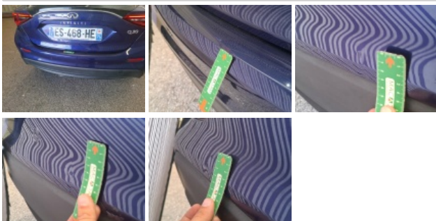
Bumper R, Deformed / Strained, Replace and paint
