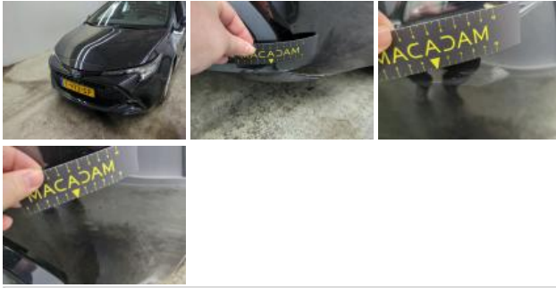
Bumper R, Scratch(es), Repair and paint (complete)
