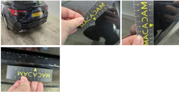
Bumper R, Scratch(es), Repair and paint (complete)
