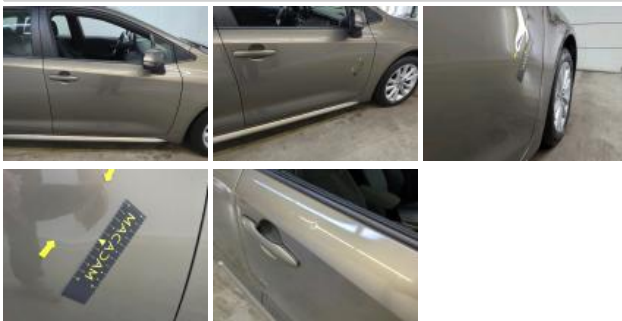
Wing FR, Dent(s), Repair and paint (complete)
