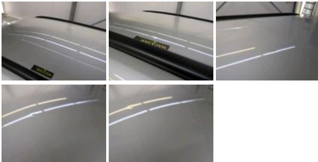
Roof, Hail damage, Paintless dent repair (hail)
