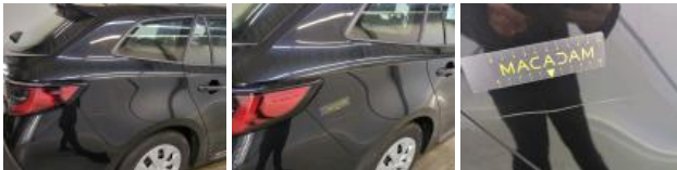
Roof pillar R, Chemical polution, Polish
