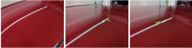
Roof, Hail damage, Paintless dent repair (hail)
