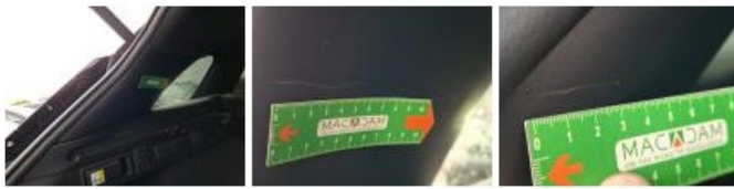
Rear bulkhead lining, Scratch(es), Repair/replace (lump sum)
