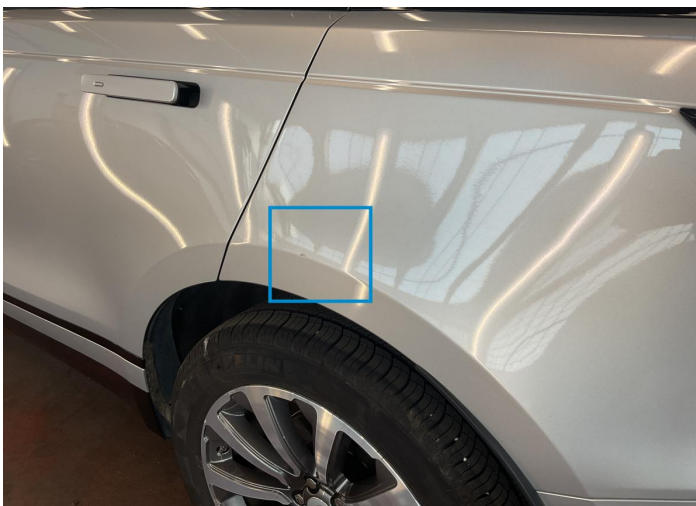
10. Fender / Back Left Bodywork / Dent -
