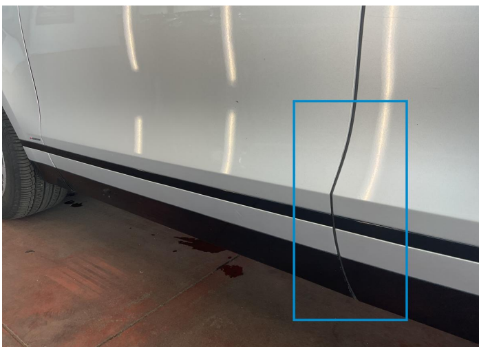
8. Door / Front Left Paint / Scratch / Line -
