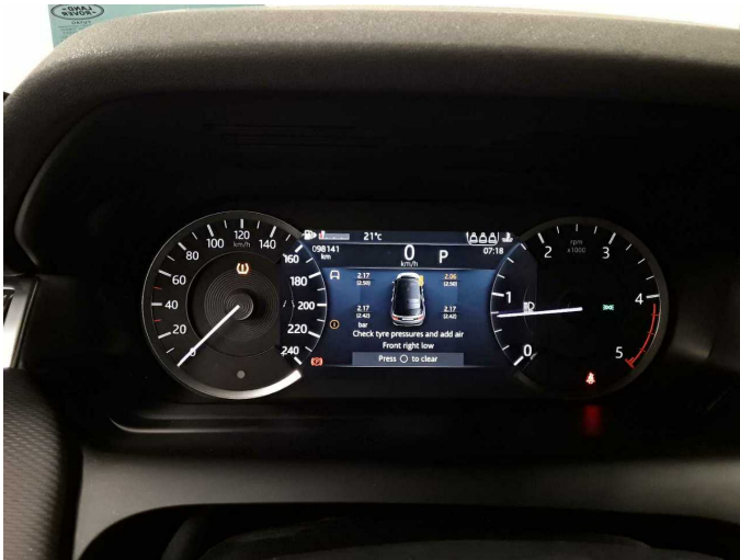
Damage 3: Instrument panel: Indicator light (Reifendruckkontrollleuchte) - on - Diagnosed and repair if necessary
