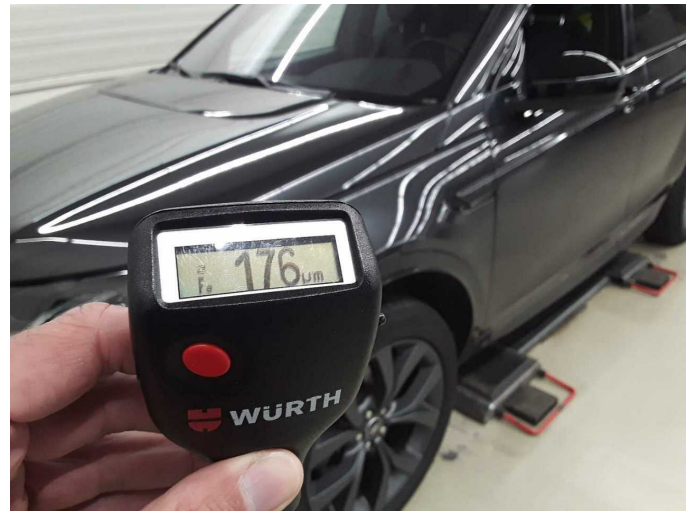
Mudguard - left side: 176 µm
