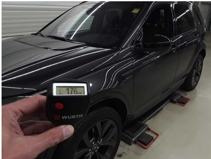
Mudguard - left side: 176 µm
