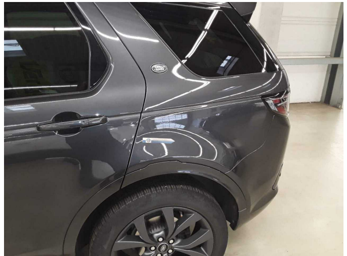
Damage 9: Side panel - rear left side: Side panel - Scratch(es) - Repair and paint
