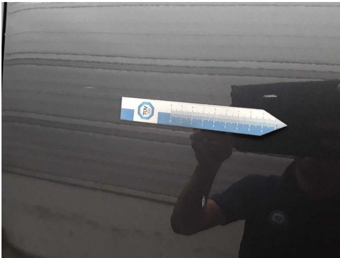
Damage 10: Door - front right side: Door - Scratch(es) - Repair and paint
