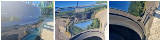
Wing trim RL, Scratch(es), Replace
