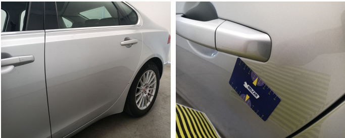
Door Rear Left // Repair & Painting-bad repair
