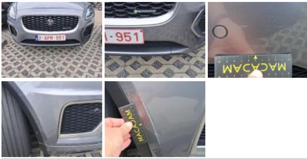
Alloy rim FL polished, Scratch(es), Repair and paint (complete)
