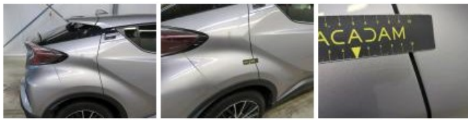
Door FR, Bad repair, Repair and paint (complete)
