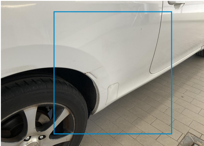
9. Side Panel / Back Right Bodywork / Breakage / Crack -
