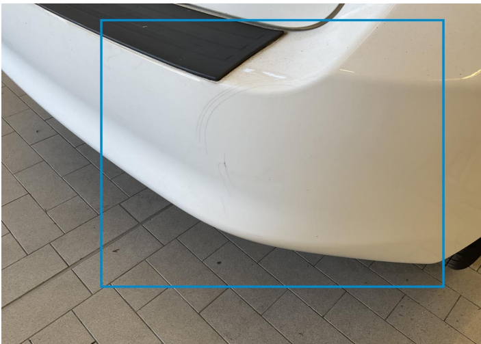
8. Bumper / Back Bodywork / Breakage / Crack -
