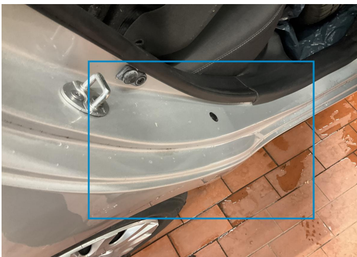
20. Pillar / Back Right Bodywork / Dent / Dent -
