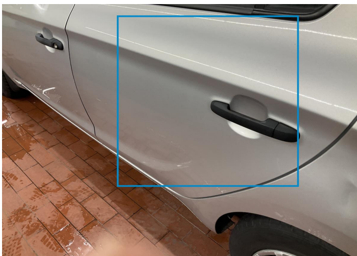
13. Door / Back Left Paint / Scratch / Scuff -
