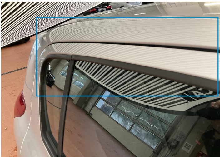
7. Pillar / Back Right Bodywork / Dent / Dent -
