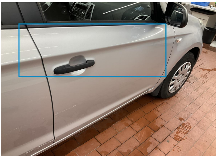
22. Door / Front Right Paint / Scratch / Scuff -
