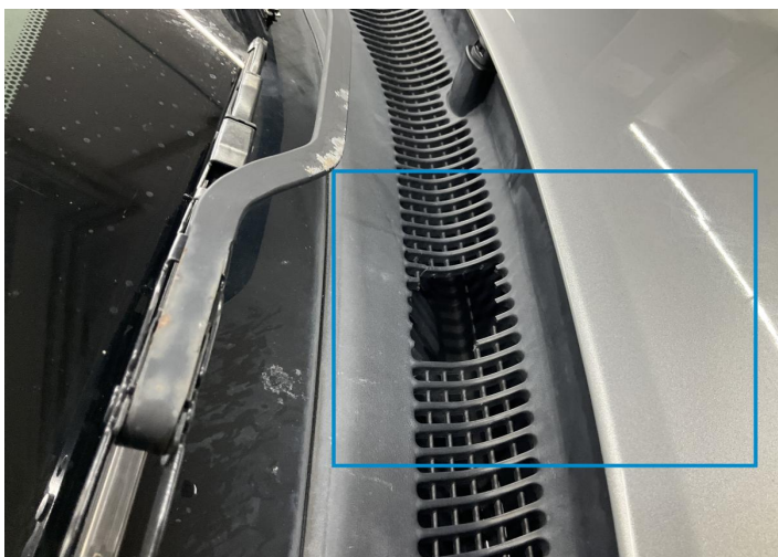
23. Hood Bodywork / Breakage / Hole -
