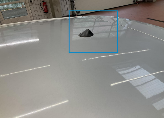
25. Antenna Rod Missing Part -
