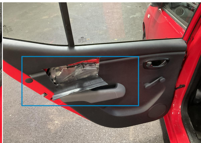
2. Panel Filling / Back Left Interior / Holed -
