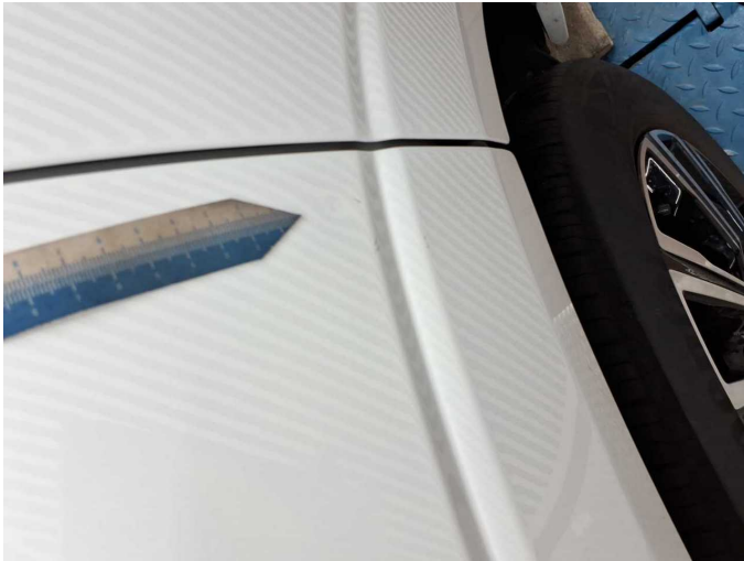
Damage 4: Side panel - rear right side: Side panel - dent(s) - Smart repair
