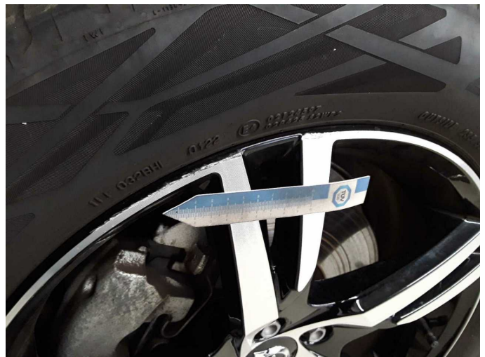
Damage 2: Wheel / tyres: Alloy rim - front left side - Scratched - Replace
