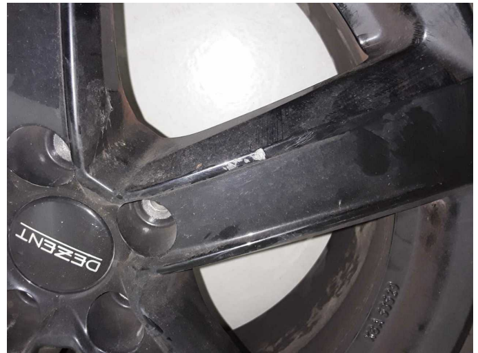
Wear and tear 4: 2nd wheel set: 1 alloy rim - Scratched - No deduction
