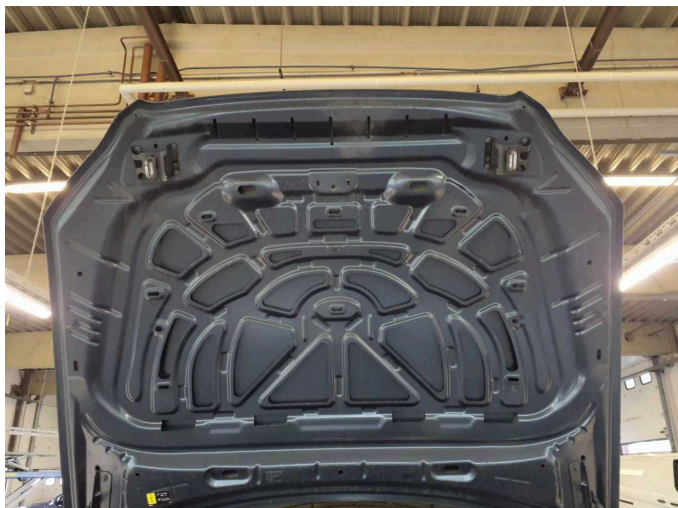
Damage 1: Bonnet: Insulation lining - Missing - Replace
