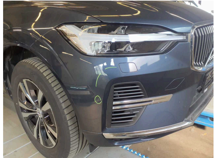
Damage 4: Front bumper: Front bumper - Scratch(es) - Paint
