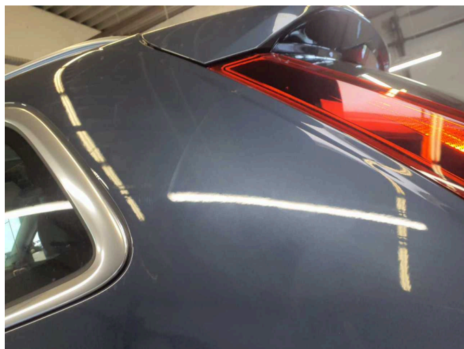
Damage 2: Side panel - rear left side: Side panel (Farbnebel+Pickel) - Unprofessionally repaired - Paint
