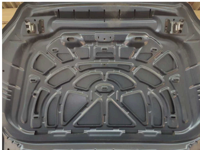
Damage 1: Bonnet: Insulation lining - Missing - Replace
