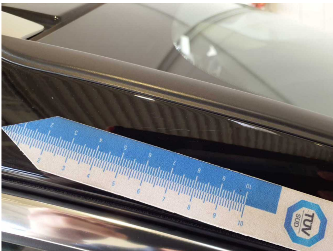
Damage 1: Roof: Roof rail - right side - Scratch(es) - Smart repair
