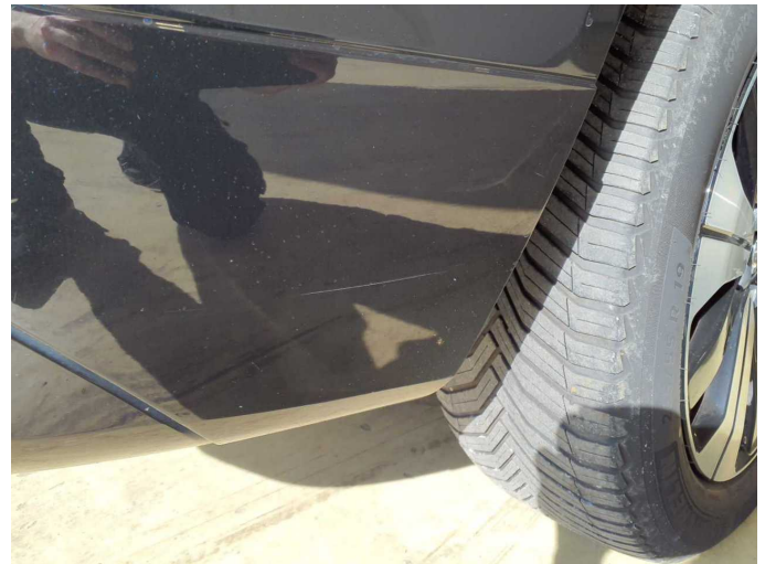
Damage 11: Rear bumper: Rear bumper - Scratch(es) - Paint
