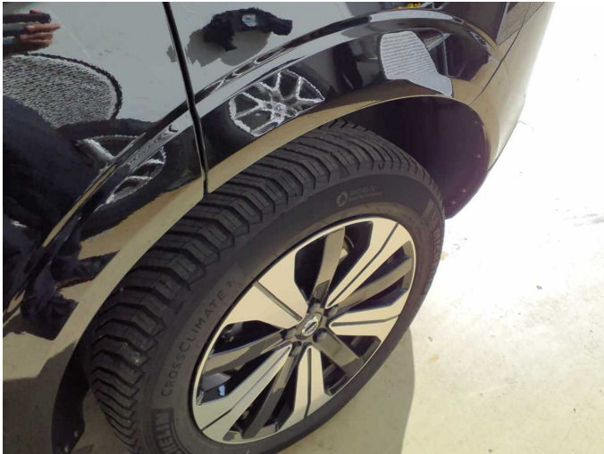
Damage 9: Wheel / tyres: Tyres - complete set - Worn - Replace
