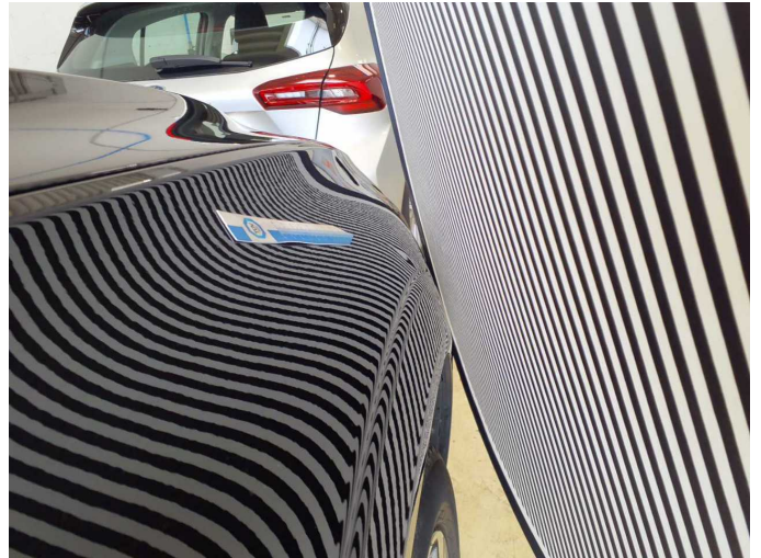
Damage 8: Mudguard - right side: Mudguard - right side (+ Steinschläge) - dent(s) - Repair and paint
