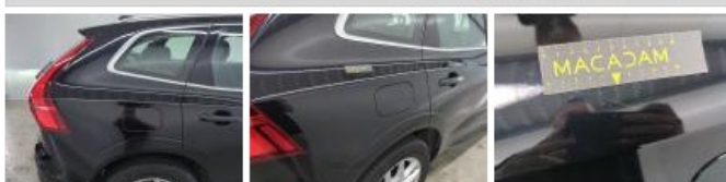
Wing RR, Scratch(es), Repair and paint (complete)
