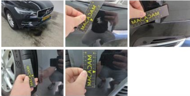
Bumper FM, Scratch(es), Repair and paint (complete)
