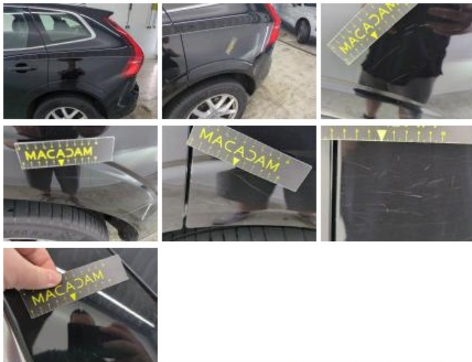
Roof pillar L, Scratch(es), Repair and paint (complete)
