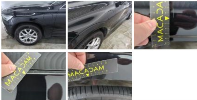
Wing RL, Scratch(es), Repair and paint (complete)
