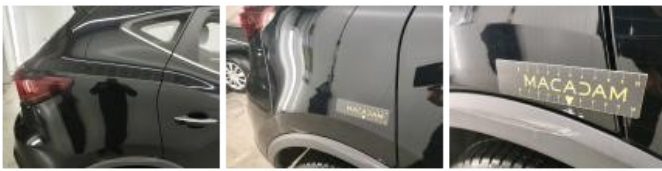
Wheel arch cover RR, Scratch(es), Replace
