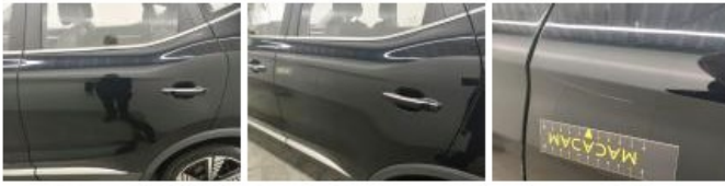
Door RL, Scratch(es), Repair and paint (complete)
