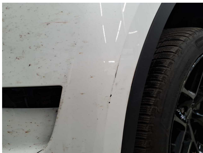
Damage 2: Front bumper: Front bumper - Scratched - Paint
