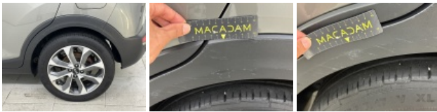
Bumper V bekleding, Gebroken, Vervangen
