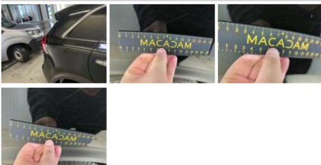
Door RR, Scratch(es), Repair and paint (complete)
