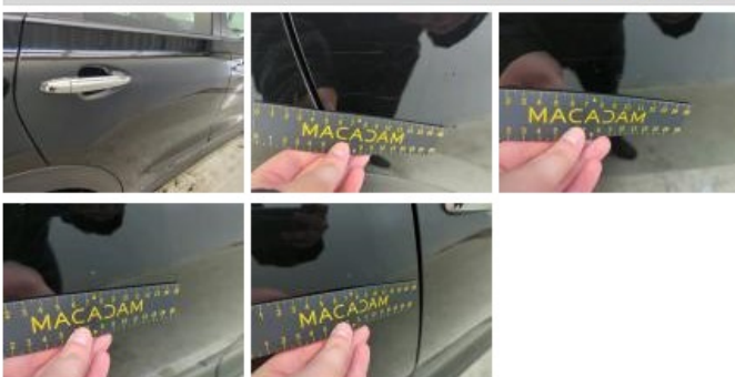
Door FR, Scratch(es), Repair and paint (complete)
