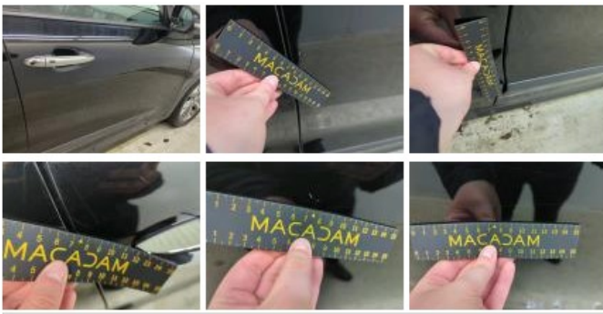
Wing FR, Scratch(es), Repair and paint (complete)
