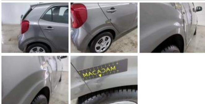
Door RR, Scratch(es), Repair and paint (complete)
