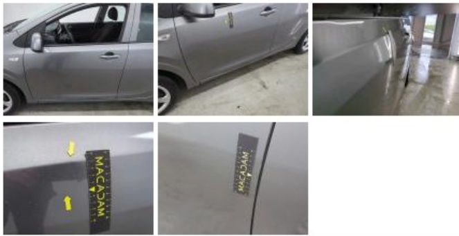
Door RL, Scratch(es), Repair and paint (complete)
