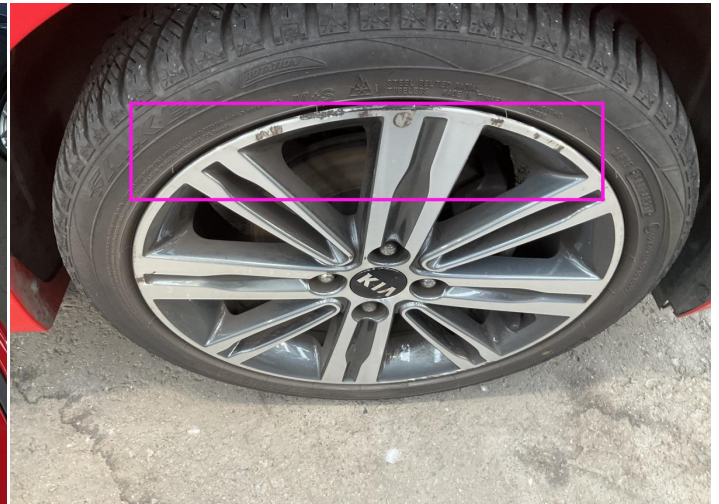
2. Rim / Front Right Out of Bodywork / Scratch -
