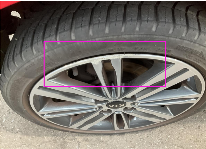
3. Rim / Back Right Out of Bodywork / Scratch -
