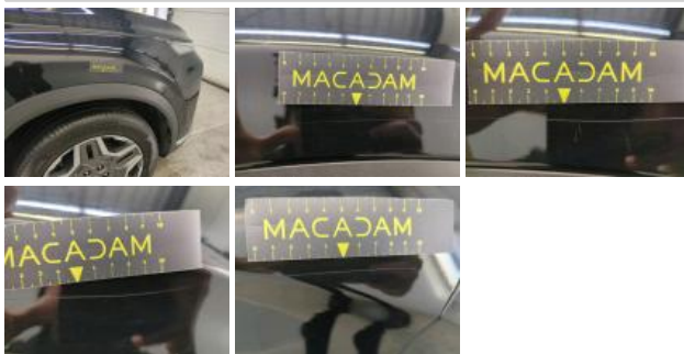
Door FR, Scratch(es), Repair and paint (complete)
