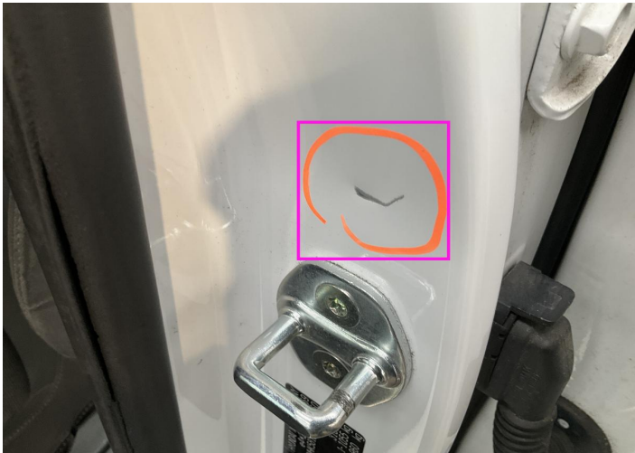
1. B Pillar / Center Left Bodywork / Dent / Dent -
