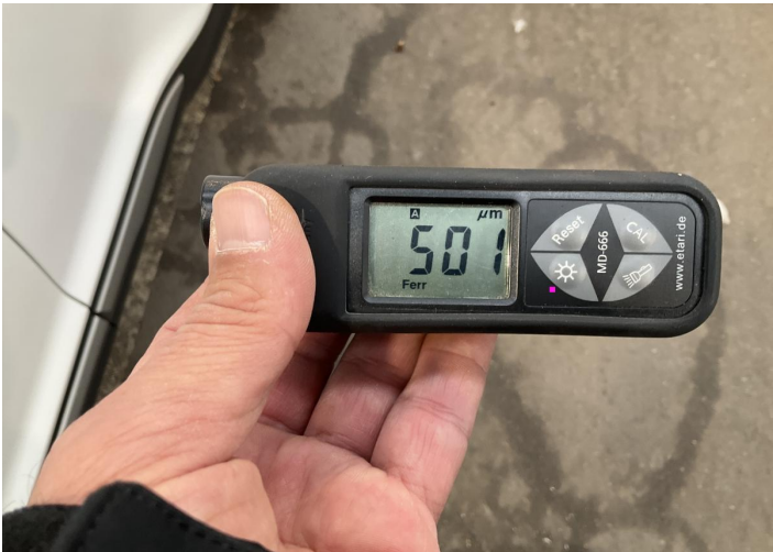
4. Door / Front Left Paint / Poor Previous Repair -
