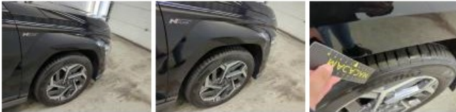
Wheel arch cover RR, Scratch(es), Replace
