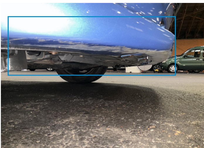
4. Bumper / Front Paint / Scratch / Scuff -
