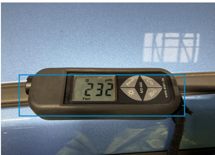
11. Door / Front Left Paint / Poor Previous Repair -
