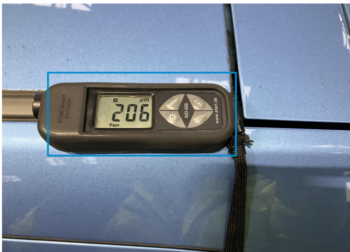
15. Door / Back Left Paint / Poor Previous Repair -
