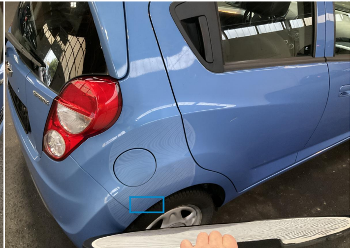
26. Side Panel / Back Right Bodywork / Dent / Dent -
