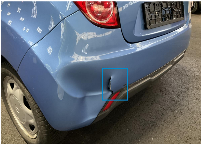
21. Bumper / Back Bodywork / Breakage / Hole -
