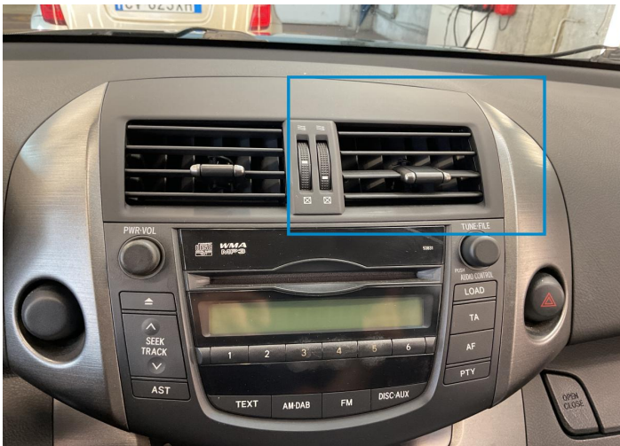
1. Aeration Grid / Front Center Interior / Broken -
