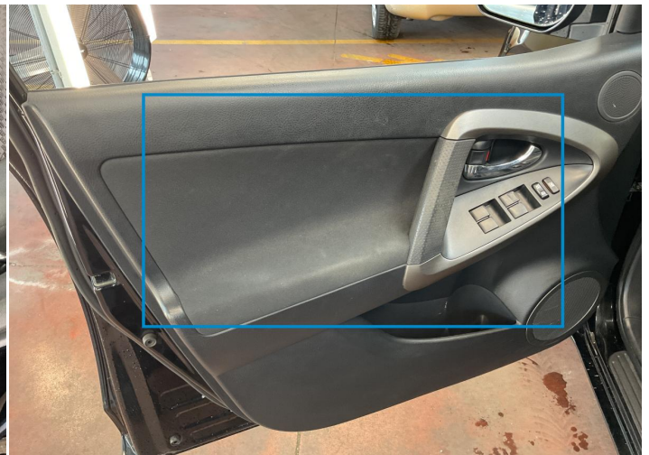
4. Panel Filling / Front Left Interior / Worn - out -
