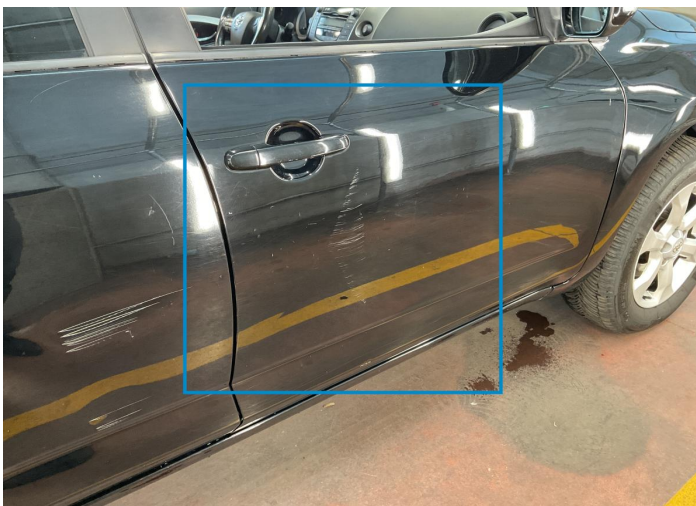
22. Door / Front Right Bodywork / Dent -
