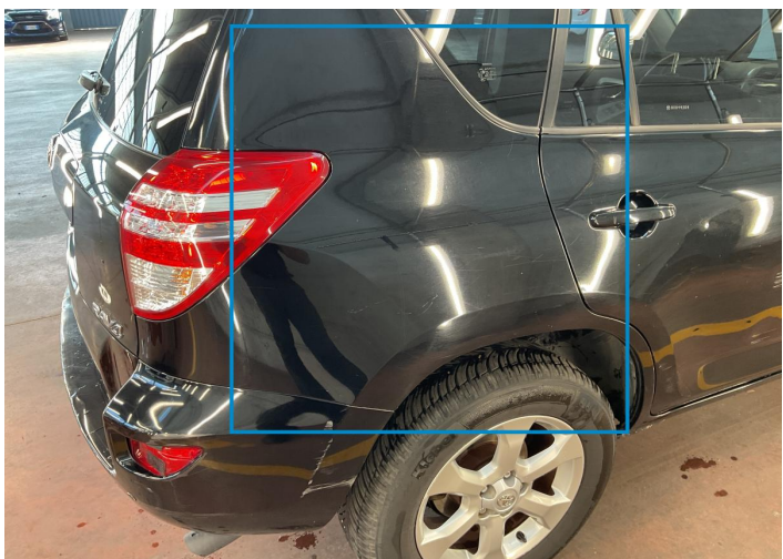
19. Fender / Back Right Paint / Scratch / Line -
