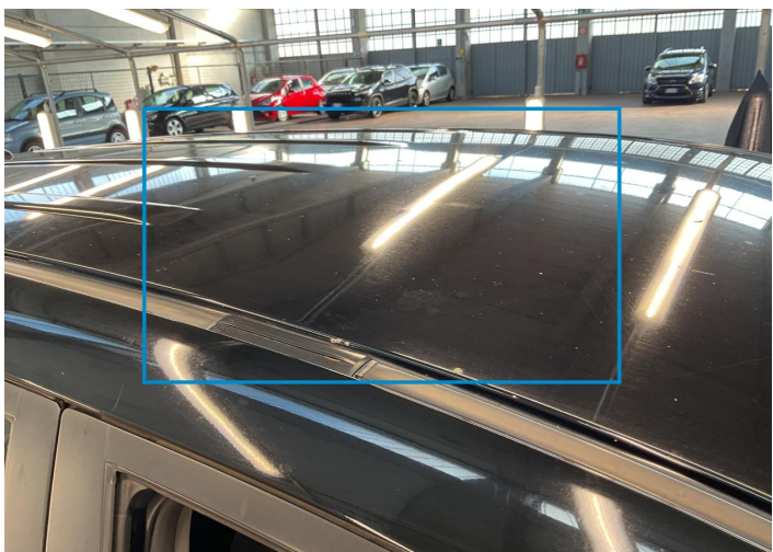
23. Roof Bodywork / Dent / Hail Area -
