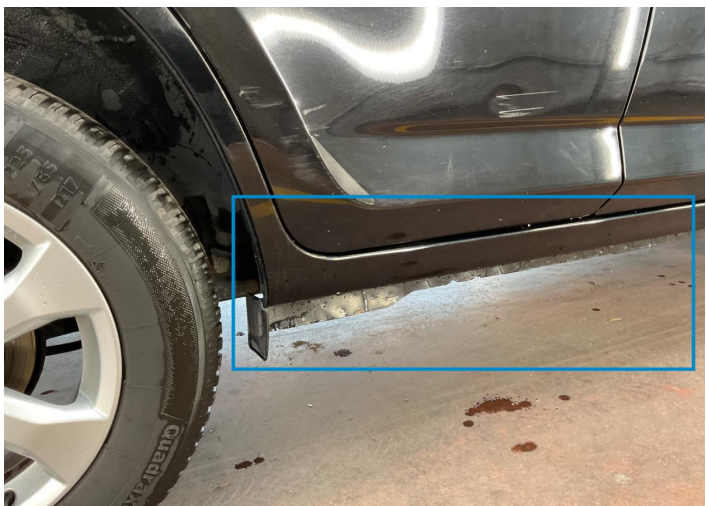
21. Rocker Panel / Center Right Bodywork / Dent -
