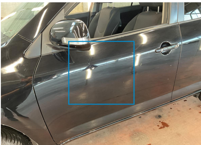
12. Door / Front Left Bodywork / Dent -
