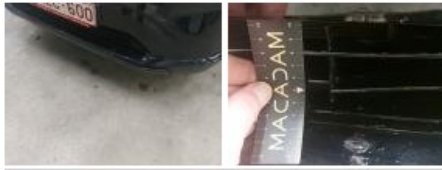
Bumper moulding F, Dent(s) and scratch(es), Repair and paint (complete)
